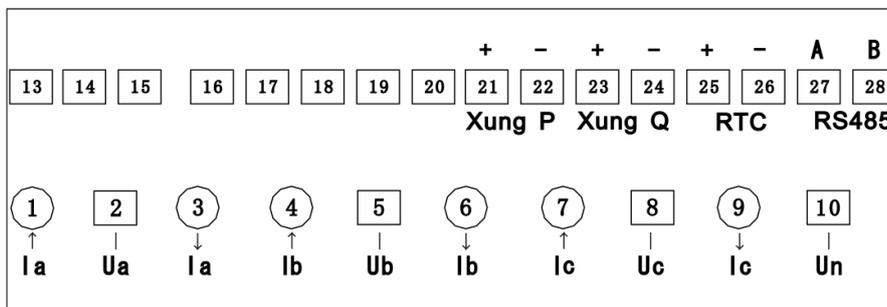
**Notice:** For VSE3T-50 type, combine voltage bridge when wiring (not applied for VSE3T-5 type)
