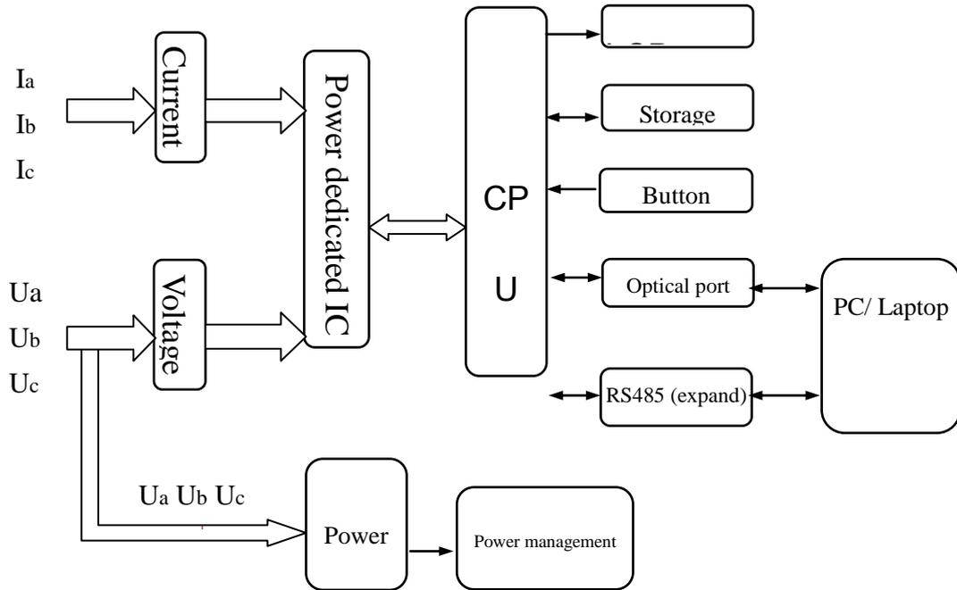
Figure 1: Schematic of working principle.
