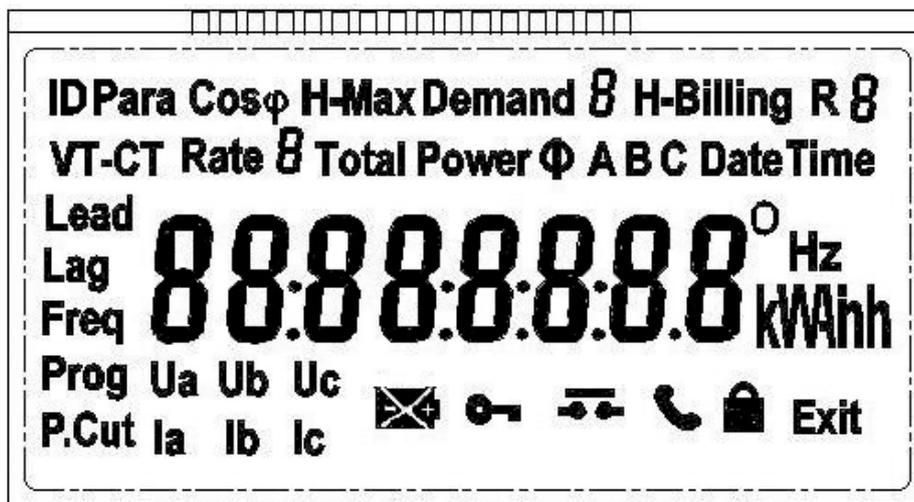
2.1. After supplied power, meter will start in 3 seconds (LCD display full content), after that, meter display the parameters in the automatic mode (these parameters can be set ). Time interval between the parameters displayed can be programmed from 1 second to 60 seconds.
